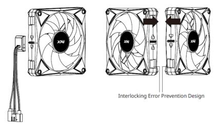
3. With an additional Fan-to-Fan extension cable, you can easily adjust your fan connection to suit any scenarios you want.
