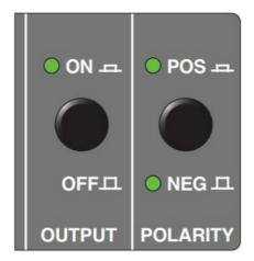
It is possible to remote control the polarity change of HCP models that are equipped with an analog programming or digital interface.
