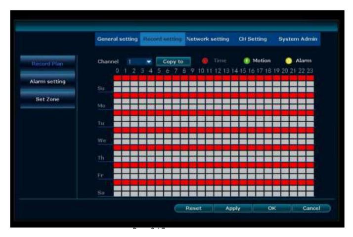
Note: This is NVR default record-setting, it means the NVR will record 24/7 continuously.
