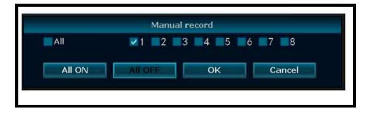
**Note:** Manual recording has the highest priority, which means once manual recording is ON, NVR will record 24/7, even though you set the motion recording at the same time.
