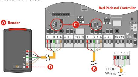
A Main Reader – The main reader is mounted at the door with a 22/5 or 22/6 wire ran to the door controller. Wire the reader to the controller as shown above. Be sure to check polarity and voltage prior to powering the controller. B Secondary Reader – Wire the second reader to the controller as shown above. Be sure to check polarity and voltage prior to powering the controller.
