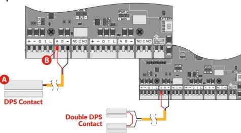
**A DPS (Door Position Switch)** – The DPS is mounted on the door frame in the desired location with a 22/2 wire running from the DPS to the controller. Wire the DPS to the controller as shown above. When using two DPS sensors for double doors, you will wire them in series with only two conductors running back to the controller for connection.
