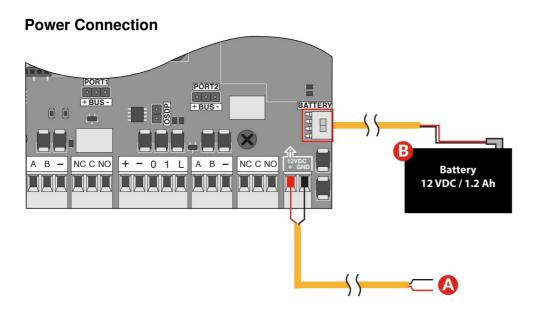
**A DC INPUT** – Use included 14 VDC, 2 Amp transformer for DC power input. It is recommended to use 18/2 wire. For high voltage applications, use the HV Converter (PN: HVC).
