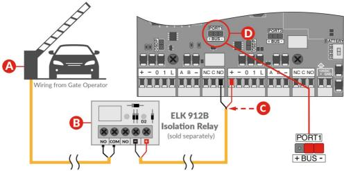
**A Gate Operator** – Follow the gate operator wiring instructions to connect the gate operator to an ELK 912B Isolation Relay.
