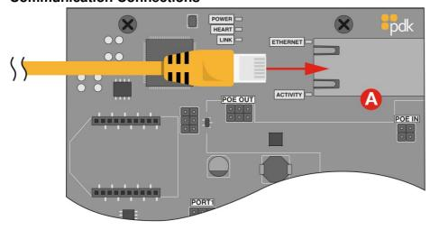
**A Ethernet** – All Red controllers come with a built-in RJ45 connection for network connectivity. Once connected, the Red Pedestal controller is Self-Discoverable from pdk.io using IPV6. Alternatively, you may use IPV4 or assign a static IP using pdk.io if desired.
