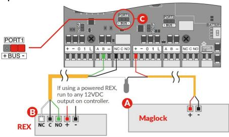
**A Maglock** – When installing a Maglock, it is typical to install a REX (Request to Exit) at the door for free egress. Run an 18/2 wire from the Maglock to the door controller, connecting to the Maglock as shown.
