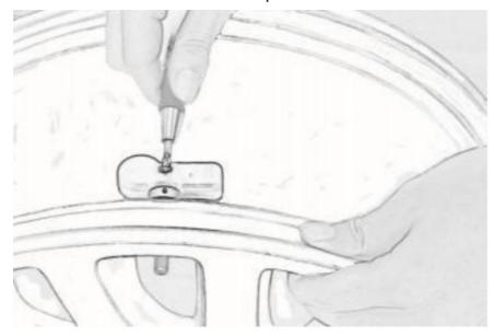
3. **Step 3:** Tighten the air nozzle fixing nut with a wrench to complete the installation. Note that the wrench uses a torque of 7 N•m.
