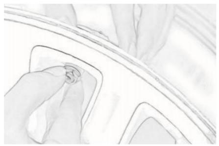
2. **Step 2:** Fix the sensor on the air nozzles with the sensor fixing screw. Note that the sensor should be close to the hub with a torque of 4N•m.
