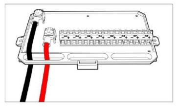
Connect the included power and ground wires. First, connect the wires to the XKcommand hub. PLEASE NOTICE THE WIRING DIAGRAM ABOVE. The RED power wire connects to the terminal CLOSEST to the output rail. If these wires are connected wrong, the XKcommand hub WILL short and this WILL NOT be covered under warranty. Route wiring through the slotted channel as shown above. Next, ground wire to the battery. Do not connect the power wire to the battery until all output channels are wired.
