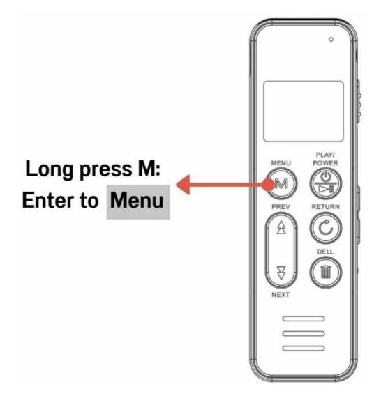
• After power on, press and hold [M] to enter menu. Short press [PLAY/OK] to save changes, short press [RETURN] to exit.
