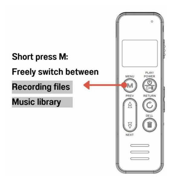
• After power on, short press [M] to switch between recording/music files. This function is useful for you to distinguish between the recording files and music files. 9
