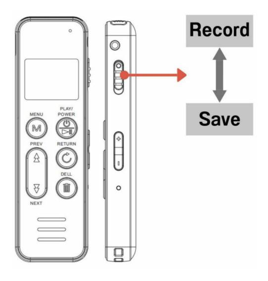
• In the power-on/off state, you can quickly record with one key. 8
