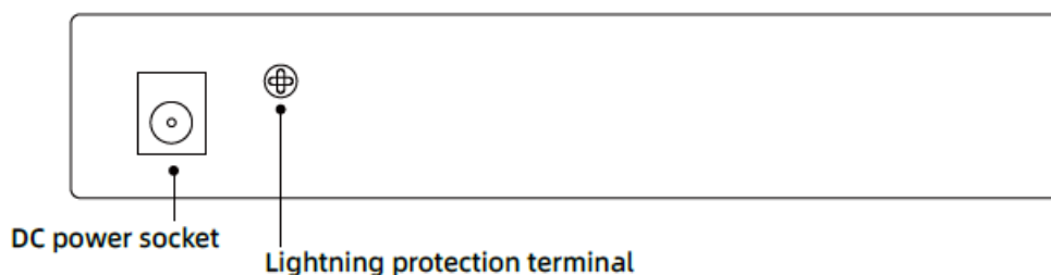
Figure 1-2 rear panel of the switch
