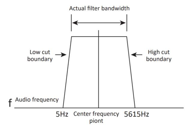
As shown in the figure on the right, the filter consists of L-CUT and H-CUT, and both work together to form an effective filter bandwidth.
