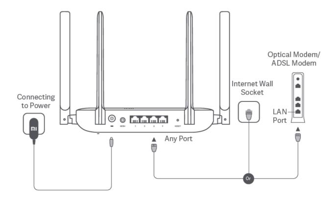
• Power on the router, and use the network cable to connect any port on the back of the router to the LAN port of the broadband modem.
