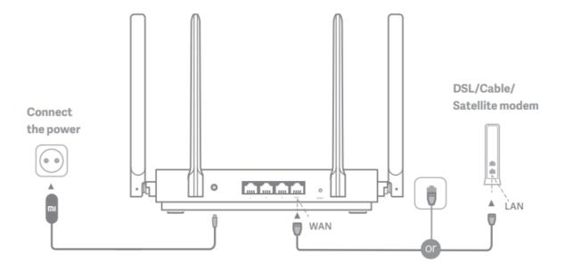
Power on the router, then connect the Internet (WAN) port to the DSL/Cable/satellite modem
