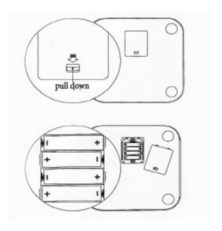
On image, which is below, shown how to open unit cover for the battery. Then place 4 batteries in the unit. Pull down the button cover
