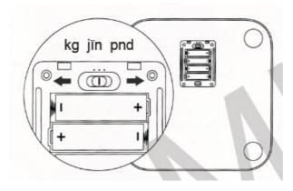
You can adjust and set required unit for weight measurement by moving to the right, left, Mi scales can measure weight in kg, jīn and pounds.
