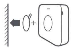
• c. Hanging: Remove the back cover of the monitor, and lead the lanyard's loop through the hole and around the hook. Reinstall the back cover, then hang the monitor.
