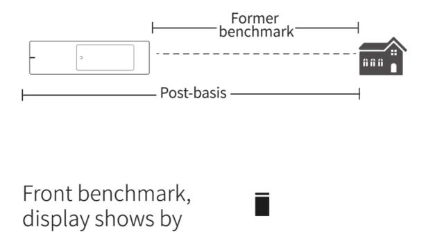
• Front/Back reference: means whether the body length is counted in the measurement data of both ways. Front datum: Without fuselage length. Back reference: Include fuselage length.
