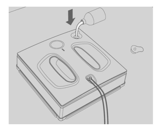
Turn on the bottom switch; attach the machine to the pane, then press the round Start button and the machine starts to dry wipe. When placing the machine, avoid being too close to the window frame. After wiping is finished, hold the secure rope with one hand and press the start button with the other hand. When the wind decreases, take down the machine and turn off the bottom switch.
