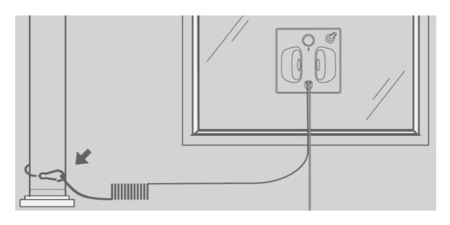
Lock the knob of the extension cable with the cable of the adapter properly. Connect the plug to the adapter, and then connect the socket to the power supply.
