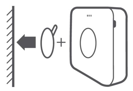
• Hanging: Remove the back cover of the monitor, and lead the lanyard's loop through the hole and around the hook. Reinstall the back cover, then hang the monitor.
