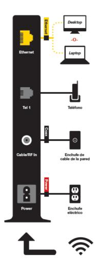
Connect the Ethernet cable from the Ethernet connection on your computer to the Ethernet connection on your Wireless Gateway.
