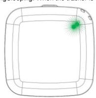
Indicator light: Flashes once per second when moving, turns off when stationary, flashes three times per second when low battery, and stays on when charging turn off when fully charged
