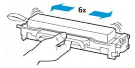
6. Remove the seal, and then remove the cover
