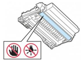
CAUTION—HOT SURFACE: The inside of the printer might be hot. To reduce the risk of injury from a hot component, allow the surface to cool before touching it.
