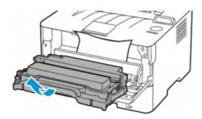
**Warning:** Do not expose the imaging unit to direct light for more than 10 minutes. Extended exposure to light may cause print quality problems.
