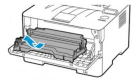
3. Remove the used toner cartridge from the imaging unit
