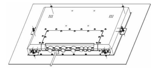
**Step 4:** Tighten the shorter M4x8mm screws to secure the bracket and tighten the longer M4x20mm screws to secure the monitor against the panel.
