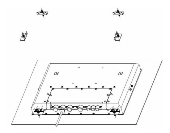
**Step 3:** Install the four remaining brackets. One on the left, One on the right, and two on top.
