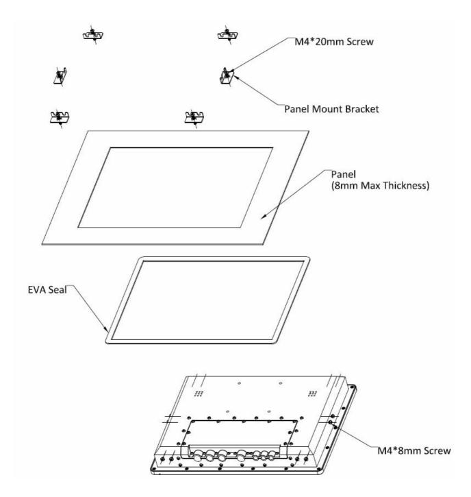
**Step 1:** Create panel cut out, place EVA seal, and install two bottom brackets.
