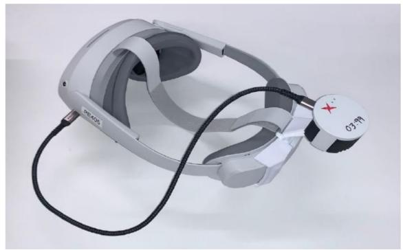
4. To charge the Host, disconnect the USB-C cable to the module and use the supplied OEM charger and charging cable.
