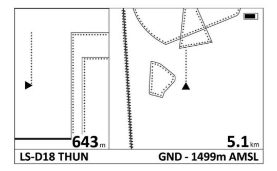
This is what the airspace screen from the Maxx II looks like when flying towards an airspace. On the left is the side view, on the right is the top view. The numbers indicate the vertical distance to the next airspace on the left, and the horizontal distance to the next airspace on the right.
