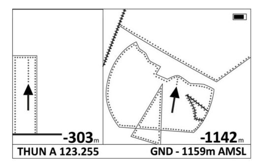
If you are inside an airspace, the two arrows indicate the shortest way out of the airspace. The displayed distance is then the vertical / horizontal distance to the airspace boundary.
