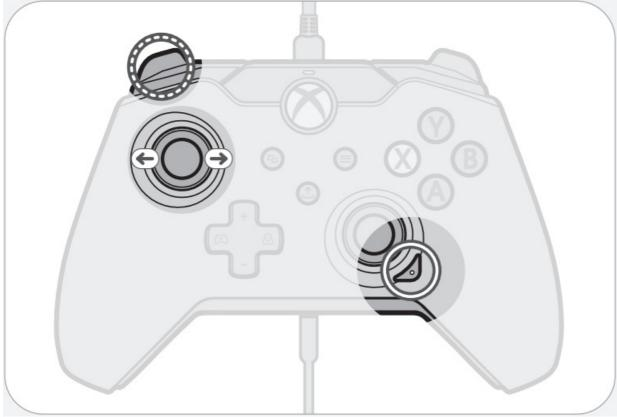
You can also adjust the brightness by holding down the "function" button and pressing the left trigger.
