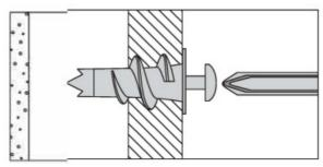
• No.3 "Cavity Fixing" wall plug minimum For use with plasterboard partitions or hollow wooden doors.
