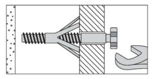
No.5 "Hammer Fixing" wall plug For use with walls stuck with plasterboard. The hammer fixing allows it to be
