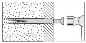
No.6 "Shield Anchor" wall plug Heavy loads For use with heavier loads such as TVV &HiFi speakers and satelite dishes etc.
