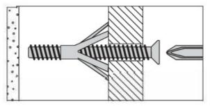
No.4 "Cavity Fixing-Heavy Duty" wall plug For use when fitting or supporting heavy loads such as shelving, wall cabinets and coat racks.
