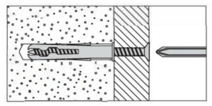
• No.2 "Plasterboard" wall plug For use when attaching light loads on to plasterboard partitions.
