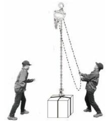
5. Never lift a load unless chain is properly seated in chain wheel(s).
