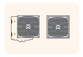
Ensure the base plate is clean & flat, and aligned with the platform.
