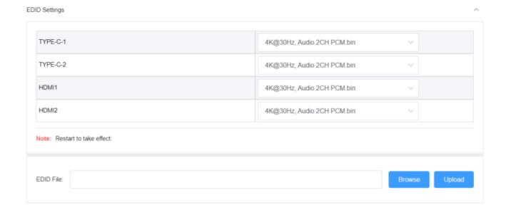
This section is used for EDID settings of input ports.
