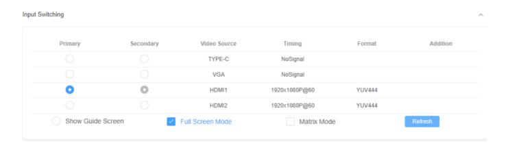
**Matrix:** In this mode, the Secondary output (output 2) can be matrix switched independently from output 1. However, when in matrix mode output 2 does not support multiview processing. Only a single full-screen input can be selected and displayed on output 2. The Primary output can still process multiview.
