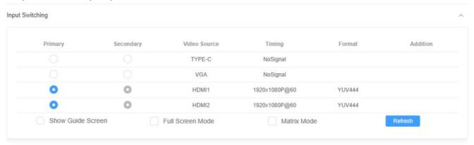
**Full Screen:** Multiview processing is not supported in this mode. Both the Primary and Secondary outputs will mirror the same content.
