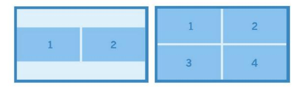
Multiview sources can be any combination of wired and wireless devices (Airplay & Miracast). For example, an iPad casting via AirPlay and a hardwired connection via HDMI can be in a split screen layout. Any combination is possible but limited to four simultaneous streams.
