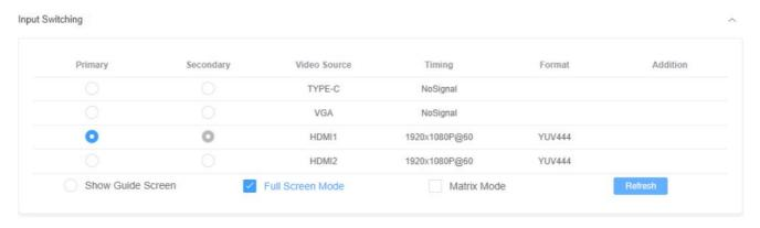
**Matrix:** In this mode, the Secondary output (output 2) can be matrix switched independently from output 1. However, when in matrix mode output 2 does not support multiview processing. Only a single full screen input can be selected and displayed on output 2. The Primary output can still process multiview.
