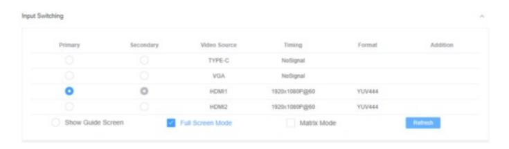
**Matrix:** In this mode, the Secondary output (output 2) can be matrix switched independently from output 1. However, when in matrix mode output 2 does not support multiview processing. Only a single full-screen input can
