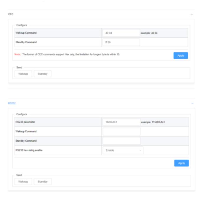
The switcher is also capable of automatically sending a power-off command after X minutes when there is no input sync detected. In the Control Strategy drop-down enter in a value between 0-60 to set how long the switcher will wait before sending the power off command. Enter in a value of 0 to disable auto standby. You can also choose what type of command is sent (CEC, RS232, or Both) during auto-sync detection.
