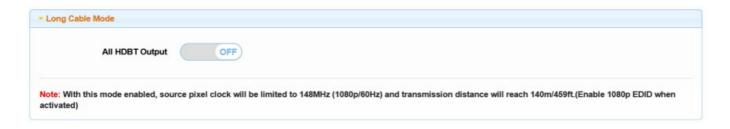
This section allows users to set long cable mode to on/off for all HDBT OUT.
