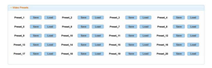
This section saves/loads the video input/output switch settings to or from the Matrix.
