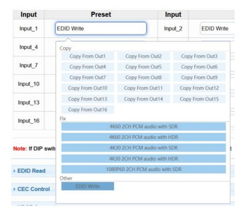
When select "EDID Write", users can select an EDID file from local PC to write it to the corresponding input port.
