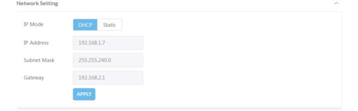
This section is to set between the static and dynamic IP address.
