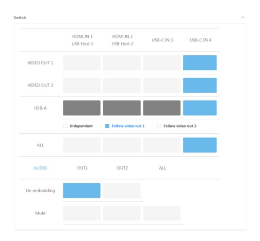
This section allows users to switch input for output, set USB-A switching, set audio switching, and mute audio.
