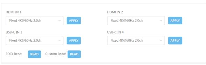
This section allows users to set EDID for inputs and read EDID of outputs. Select EDID for the corresponding input port, and click "APPLY" to take effect. Default setting for all inputs: Fixed 4K@60Hz 2.0ch. EDID selectable includes:
