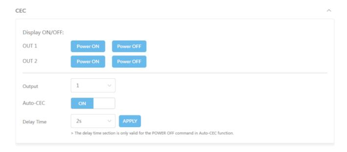
This section allows users to control the connected CEC enabled displays to power on/off, and set auto-CEC function.
