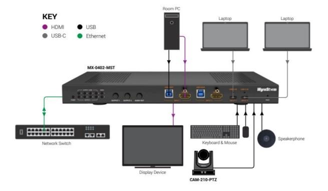
Note: By default, USB-C IN 4 is in DP SST mode, use the command "SET USBC4\_M prm<CR><LF>" to set the
