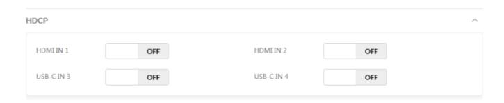
This section allows users to set HDCP function of inputs to ON/OFF. Click the button to enable/disable HDCP encryption of each input port, the default setting is "ON".
