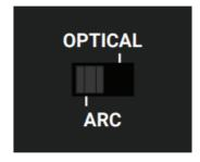
Set the audio switch to OPTICAL to send digital audio signals from the Matrix to an external AVR etc.
