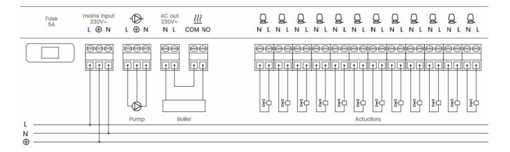
If you are wiring your two port valve or direct feed to trigger the boiler to the connection box, ensure that you select the relay within the app when you are selecting your actuators.
