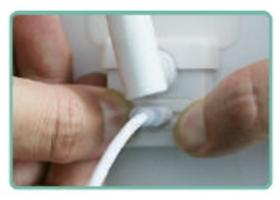
4. Please DON'T insert the charging cable directly with the rubber on the plug.
