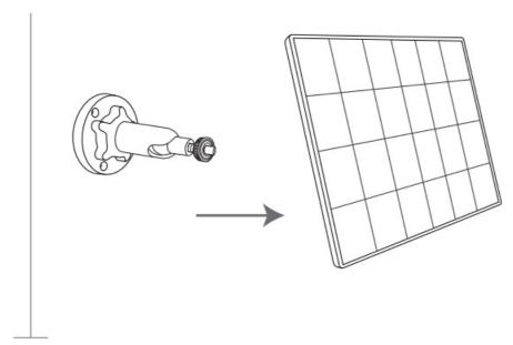
8. Align the universal joint with the Solar Panel, and lock it in place by turning the Universal Joint clockwise.
