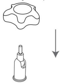
6. Clockwise spin the Locking Screw Cap.
