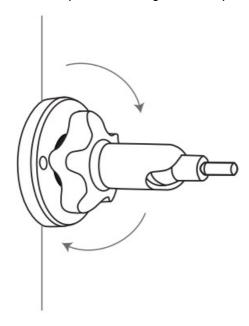
7. Then attach the joint to the back of the solar panel by screwing it in.
