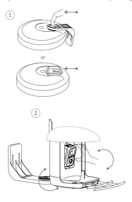
7. **Step 7**: Open the silicone plug, re-plugin the Solar Lite.
