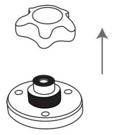
5. Slide the Locking Screw Cap into the Universal Joint until it reaches the end.
