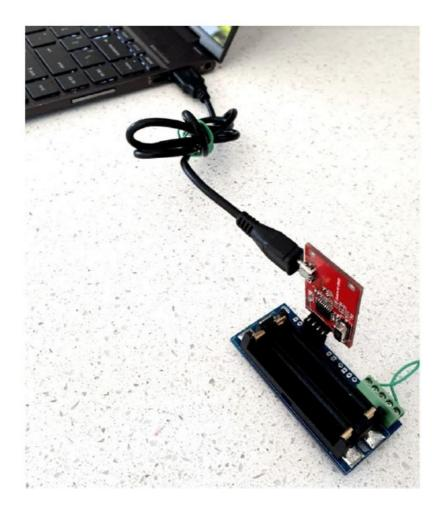
**Note:** At this moment the MReX Module will the powered and depending on the MReX configuration it should flash its green status led.
