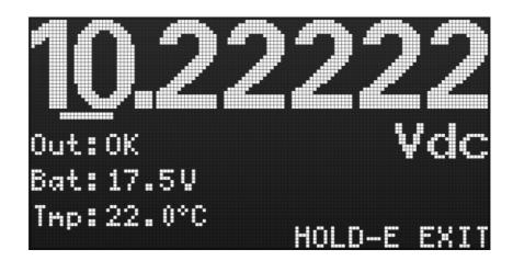
Setting an output: Use the LEFT & RIGHT buttons to select the digit you want to change then press the UP or DOWN to change the digit.
