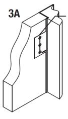
PLACE DRILL TEMPLATE ALONG EDGE OF Z-BAR WITH DOOR CLOSED, TAPE TO DOOR AND MARK HOLES.
