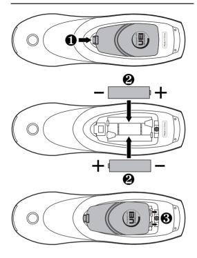
The DIRECTV® Universal Remote Control comes with preinstalled batteries. To activate them, pull the tab out of the battery case. To change the batteries, perform the following steps:
