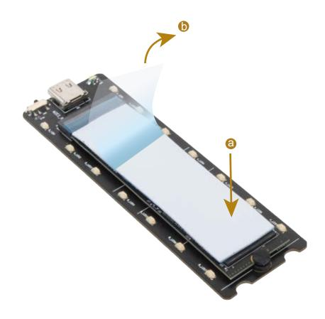
Attach the thermal pads and remove the film
