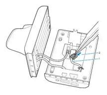
9. Reapply the sticker, ensuring it holds the new cable jack and plastic bezel in place.
