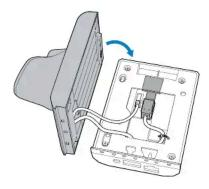
11. Secure the cup using a Philips (PH02) screwdriver. Torque to 2.55–3.45 kgf-cm (2.21–2.99 lbf-in).
