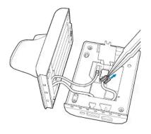
6. Disconnect the USB cable and power cable.
