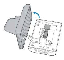
3. Using scissors, cut the cable tie and release the cable.
