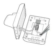
**4.** Using tweezers, lift the sticker on top of the cable connector.
