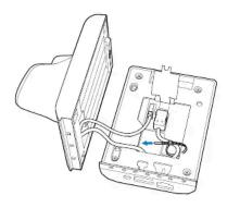
8. Position the plastic bezel between the cable (1) and the PCB (2).
