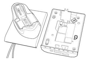
7. Connect the new cup USB cable to the connector on the base. Secure the cable to the base with a new cable tie and position it under the middle frame. Connect the power cable to the connector on the base.
