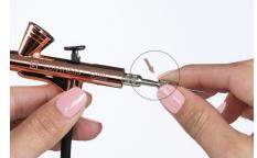
STEP 2: Loosen needle-retaining bolt; half turn of bolt is all that is necessary. Do not remove bolt all the way, just lightly loosen.
