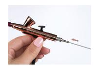
STEP 1: Return the needle back into the airbrush stylus, being careful not to bend the needle. Gently push the back end of the needle to make sure needle is firmly in place.
