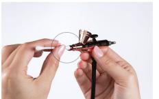
STEP 5: While the needle is out of the airbrush, clean the front nozzle with a fresh cotton swab. Remove all
