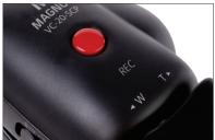
2 Use the variable-speed zoom rocker switch to control the zoom function.
