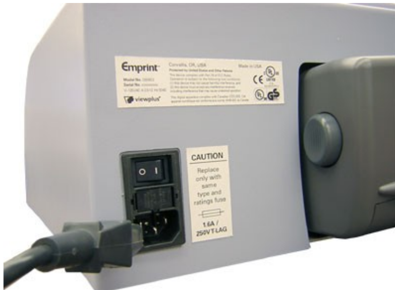
Shows the power module in the back of the embossing printer
