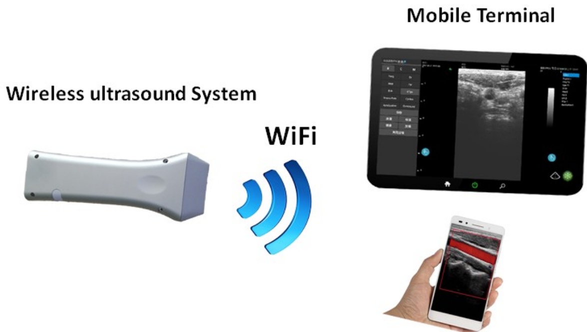
Image 2-1 Wireless Ultrasound System Working Principle
