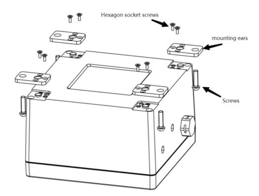
The anchor is fixed on the bracket by screws, and the bracket needs to be fixed on the vehicle by spot welding by professionals.
