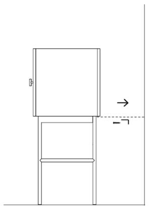
MEASURE THE HEIGHT AND DRILL HOLES IN THE WALL. APPLY SUITABLE WALL PLUGS. MOUNT THE METAL BRACKET TO THE WALL WITH SCREWS AND THEN MOUNT THE BRACKET TO THE CABINET.
