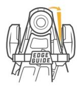
Do not put pressure onto/into the sharpening guide. It is intended to provide a reference point for blade position. Only use light pressure (weight of the blade) when using the sharpening guide to yield best results.
