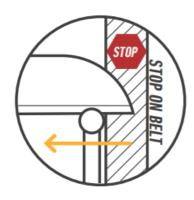
Pull straight through the guide and do not lift the blade handle as you pull. Power off as the point of the knife approaches the middle of the belt. Lift the knife up and out of the guide.
