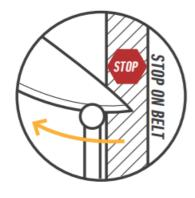
Follow the curve of the blade so the edge remains perpendicular to the travel of the belt. Power Off as the point of the knife approaches the middle of the belt. Lift the knife up and out of the guide.
