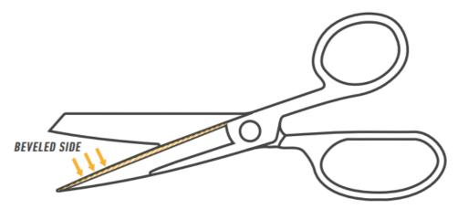
Once scissor blade is properly placed in Sharpening Guide, squeeze power switch and simultaneously pull the scissor blade steadily through the guide at 1" per second. Repeat 1-2 more times or until marker is removed from cutting edge. Repeat on other scissor blade.
