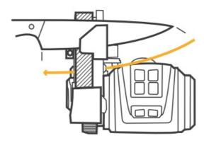
Follow the curve of the blade as you pull through the guide. Keep cutting edge perpendicular to the belt for best and most consistent results.
