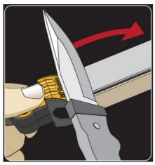
Place the side of the knife flat on the Guide closest to the handle so the cutting edge is on the abrasive and PUSH the knife edge away and along the abrasive surface.
