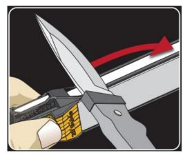
Rotate the red knob so that the fine (smooth) surface and "F" on the knob are up.
