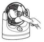
• Be sure to tighten the screws to reinstall the front grille.
