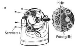
• Insert clean out any trash or debris with a vacuum cleaner. Wipe with a soft and dry cloth where the vacuum can not clean.
